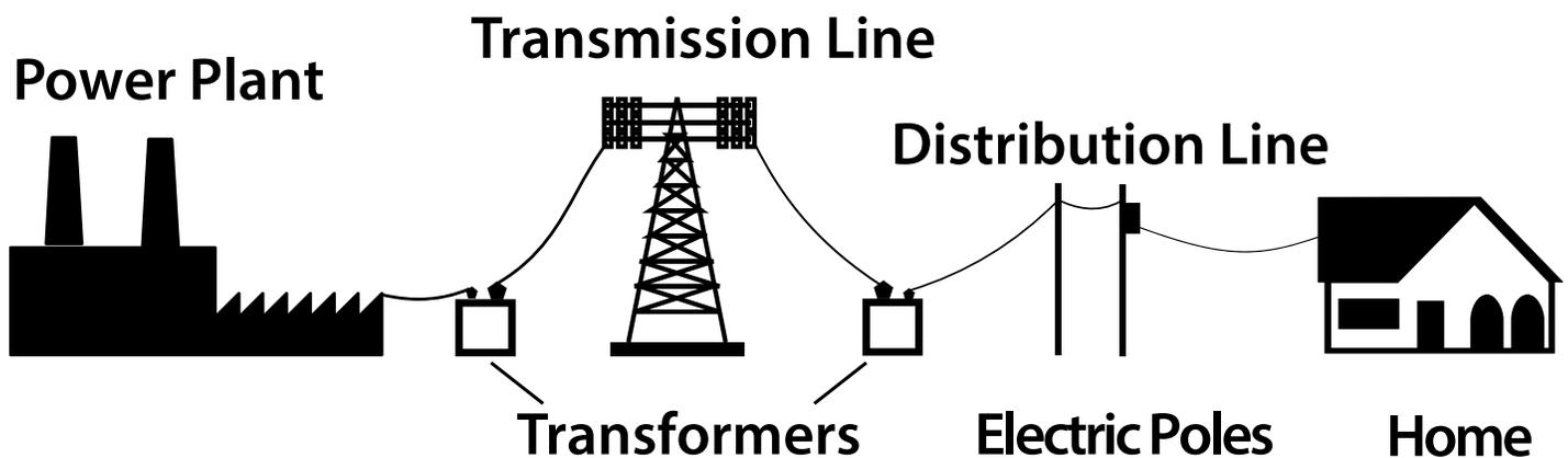
There are many different types of power lines. The power plant makes electricity. The electricity flows through **transmission lines** held up by **power towers**. The transmission lines carry large amounts of electricity to electric poles in cities and towns.
