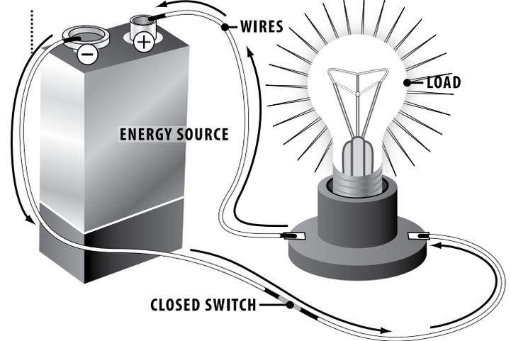
A closed circuit is a complete path allowing electricity to flow from the energy source to the load.
