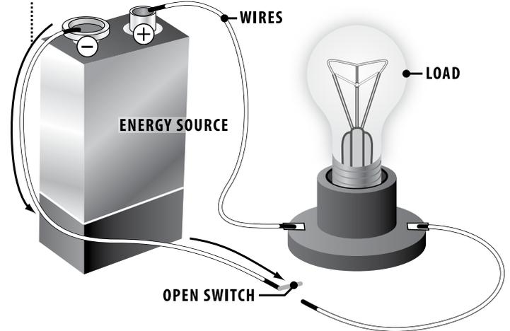
An open circuit has a break in the path. There is no flow of electricity because the electrons cannot complete the circuit.
